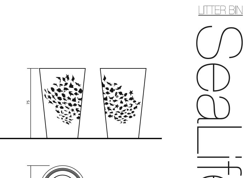
are reinforced internally with two types of glass fibre, thickness 04 and 018. To give greater strength to the shape a polyester resin and natural quartz compound is applied. The surface of the products is polished or matt on request.
