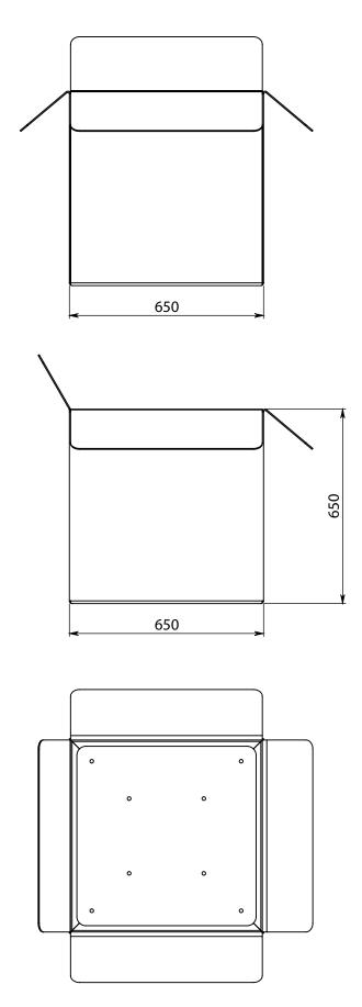
The BOX planter is in galvanised and polyester powder coated steel (or Corten treated with an oxidation cycle), thickness 40/10. On the bottom part there are 2 overflow holes made of steel tubulars
